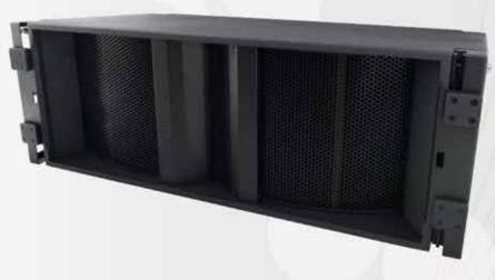
High-Power 3-way tri-amp enclousure 2 x 12-inch-LF cone Horn-Loaded / 1 x 12-inch MF cone Horn-Loaded / 2 x 1.4-inch exit HF both waveguide attached CD horn
